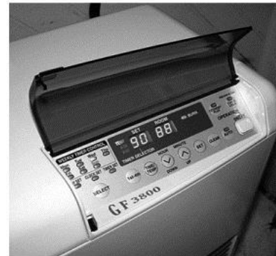
Space heater controls: Many modern energy-efficient space heaters have programmable thermostats as standard features.
