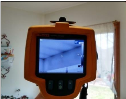
Infrared scanner: Allows the user to see temperature differences, which verify insulation coverage in a wall cavity.
